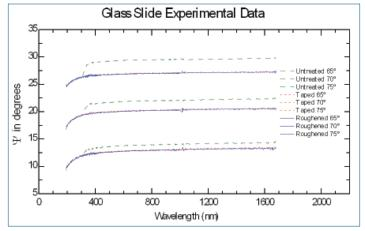
Figure 2. Ellipsometric  $\Psi$  data acquired on a glass slide. Note the slide is absorbing below 300 nm so all three data sets are identical. Beyond 300 nm the untreated slide data show backside reflection effects. Note the taped and roughened data are effectively identical.
